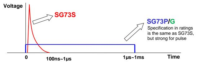
The KOA SG73S-series is a special anti-surge resistor which is suitable for high peak voltages with short duration (e.g. ESD / CR discharge / rush current, etc.)
